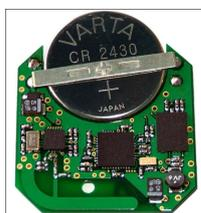
**Note:** Please ensure the positive plus sign on the battery matches the positive plus sign on the battery holder.
