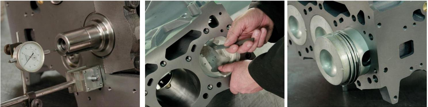
Each short motor goes through rigorous checks at both the manufacturing and assembly phases, ensuring that each component fits to the cylinder block in line with the original engine tolerances.
