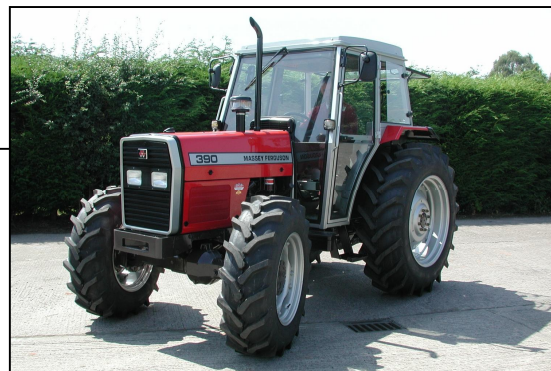
Massey Ferguson 390 uses A4.248 replacement (VPB8030)
