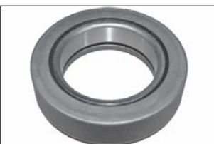
5 VPG5501 30208100, 30208110 • Type Flat faced thrust bearing • ID 60 mm • OD 96.7 mm • Height 26 mm
