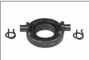
5 VPG5006 • Type Carbon in integral carrier • ID 38.2/41.5 mm • OD 76.5 mm • Height 21 mm
