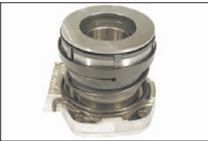
5 VPG5085 31597300, 35651700 • Type One bearing on integral slave cylinder • ID 45.50 mm • OD 95 mm • Height 105 mm
