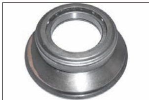
5 VPG5260 725160 • Type Flat faced thrust bearing • ID 55 mm • OD 102.5 mm • Height 29.5 mm
