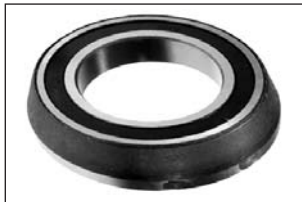
5 VPG5006 • Type Carbon in integral carrier • ID 38.2/41.5 mm • OD 76.5 mm • Height 21 mm
